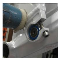
▲ Step 3: With both bolts slackened, and standing on the driveside of the bike, tap the swingarm away from you. Note: When tapping the frame always hit the weld to avoid damage.
