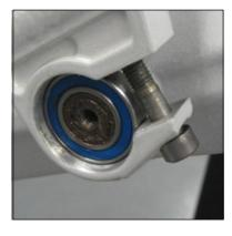
▲ Step 2: Undo the bearing clamps, remove both blocks and replace the bolts
