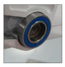
▲ Step 9: Apply copper grease to the inside of the bearing race. Centre the bearing over the pin and inside the swingarm clamp.
