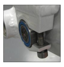
▲ Step 4: With the swingarm moved across on the bearings, tighten the clamp on the driveside of the bike.
