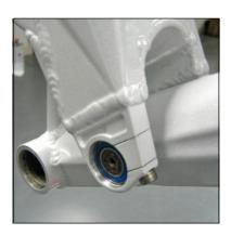
▲ **Step 1:** Using a 3mm allen key, remove the bearing end caps.
