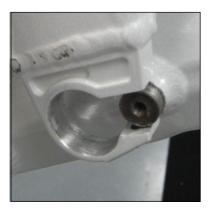
■ Step 7: If you need to remove the swingarm, slide it backwards so the pin passes through the gap.
