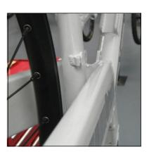
▲ Step 11: Replace clamp blocks and bolts. Centre the swingarm and tighten.
