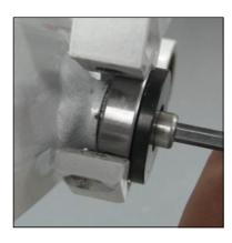
▲ Step 10: Add loctite and tighten the bearing cap over the bearing, ensuring it seats correctly as it's drawn completely onto the pin.
