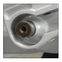
▲ Step 6: If steps 3-5 have not completely drawn the bearing off the pin, repeat the process until completely removed.
