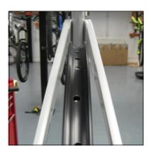
■ Step 12: Fit a wheel and check you've centred the swingarm correctly. Check alignment from the rim to seattube and shock mounts.
