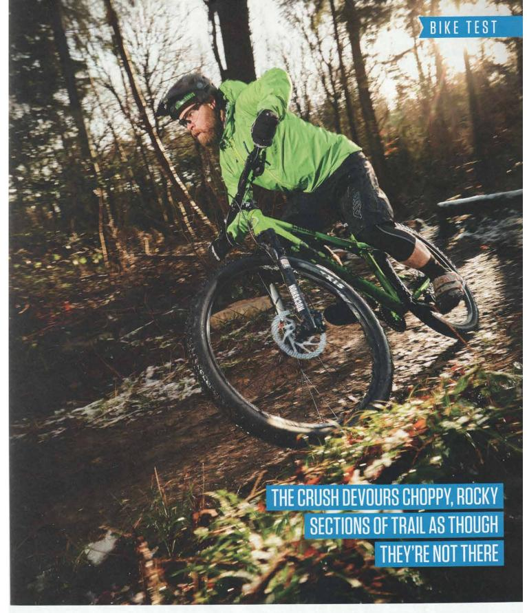
cross-country biased trail bikes is in the fork – and it's the fork that's the Crush's secret weapon. Ride with your weight forward, hovering over the saddle, and the Revelation's accurate steering and implacable rock-swallowing ability allow the Crush to devour choppy, rocky sections of trail as though they're not there. The rigid rear end keeps up a constant chatter of trail feedback at slow to middling speeds without
