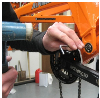
▲ Step 6: When the bolt head is out of reach use your Allen key to continue tapping the axle.
