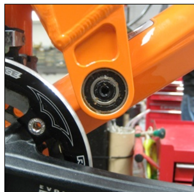
▲ Step 4: Using a 5mm Allen key, remove the bearing caps to expose the bearings.
