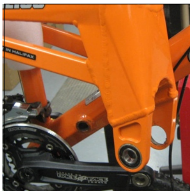
▲ Step 8: Remove swingarm, being careful not to lose the washers inside the swingarm.
