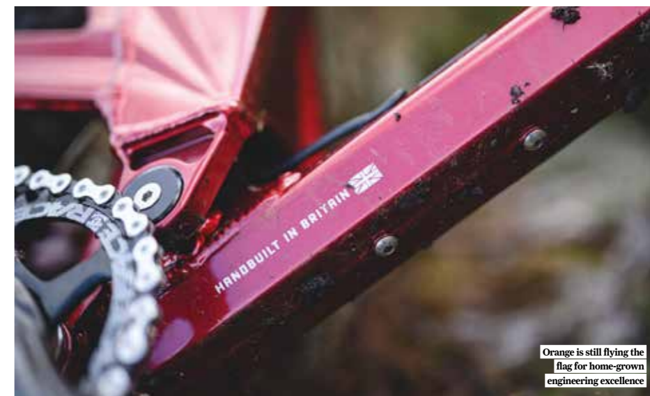
Variable-thickness alloy frame boosts vertical stiffness
